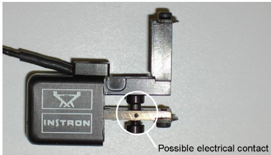
**Figure 12.** Illustration of the extensometer used. The possibility of electrical contact is highlighted.
