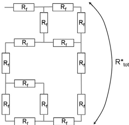
**Figure 2.** Representation of the result of damage in carbon fibre resistor network.
