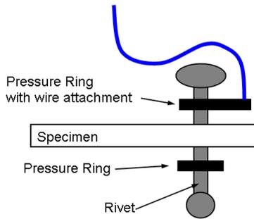
**Figure 5.** Mounting a rivet through the specimen.
