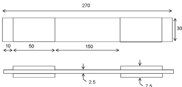
**Figure 3.** Dimensions of the tensile coupon used, equipped with isolating tabs of  $[\pm 45^\circ]_{2s}$  glass fibre epoxy.
