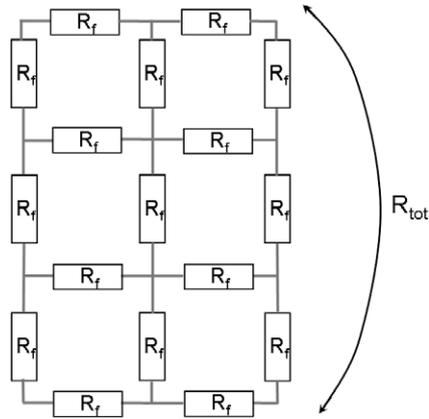
**Figure 1.** Electric network of resistors, representing a fabric of carbon fibres in an insulating matrix.
