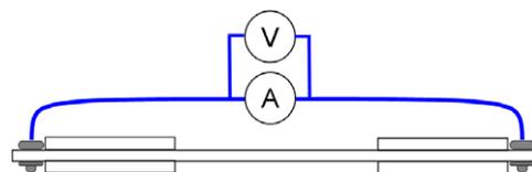
**Figure 4.** Symbolic representation of the two-probe method used for electrical resistance measurement.
