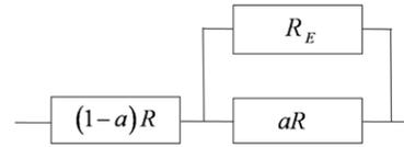
**Figure 13.** Theoretical illustration of the effect of the extensometer on the resistance measurement.
