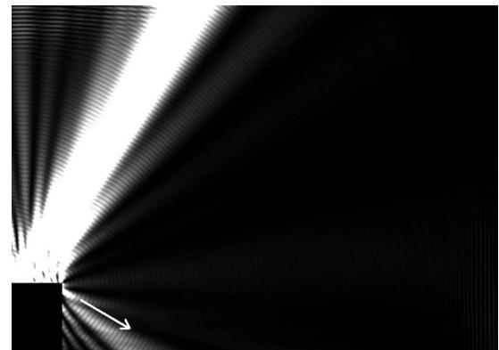
FIG. 19. Internal generation of the Rayleigh waves in an aluminum plate.
